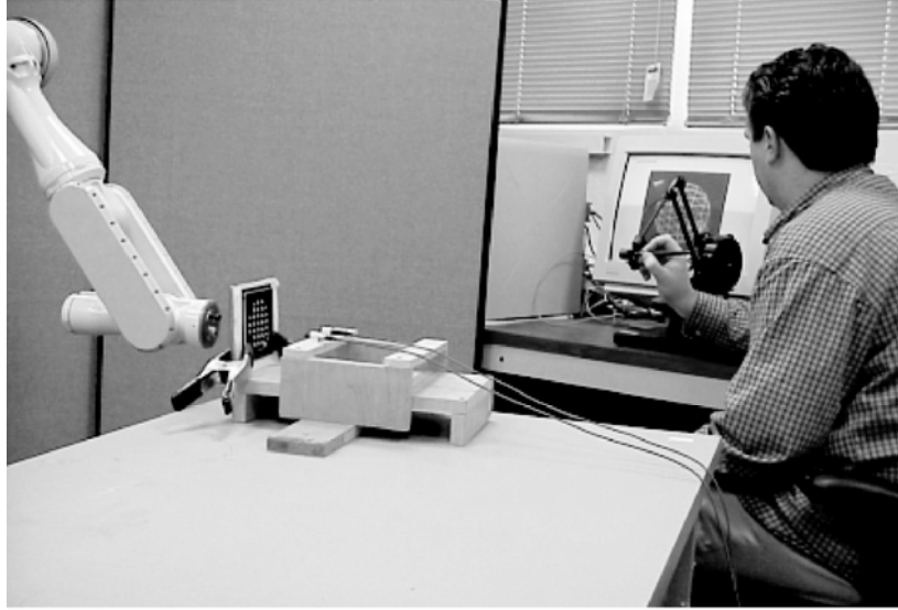
Figure 2. The experimental system for vision-based force feedback from the membrane
