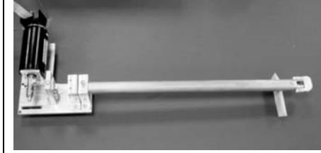
Fig. 2. Prototype of the laparoscopic grasper with force feedback.
